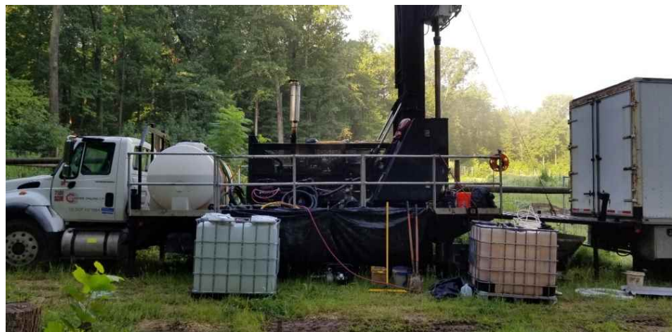
Sonic Drill Rig during VAP Sampling
