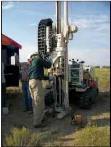
Coring for solid-phase sampling
