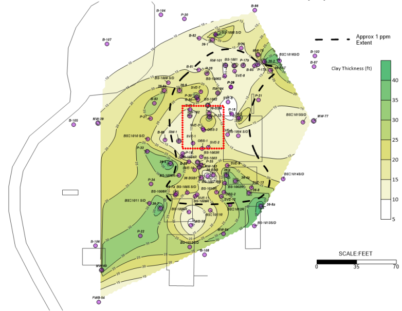
SWMU 36 ESTIMATED THICKNESS OF CLAY (FT)
