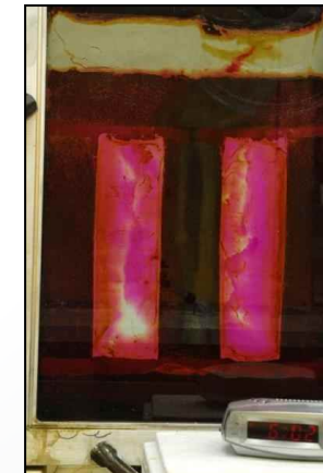
T = 12 hr w/ 8-hr EK ( \text{MnO}_4^- flushing with EK )
