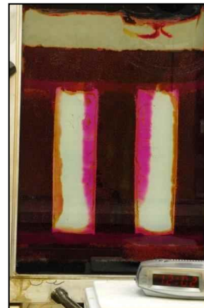
T = 6 hr w/ 2-hr EK ( \text{MnO}_4^- flushing with EK )
