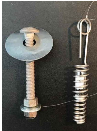
Waterloo Membrane Sampler (WMS)
