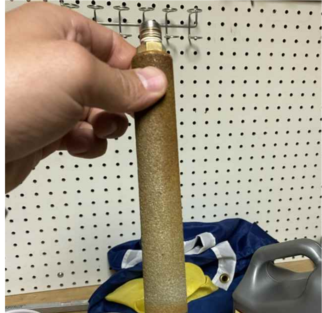
After Diffuser Cleaning
