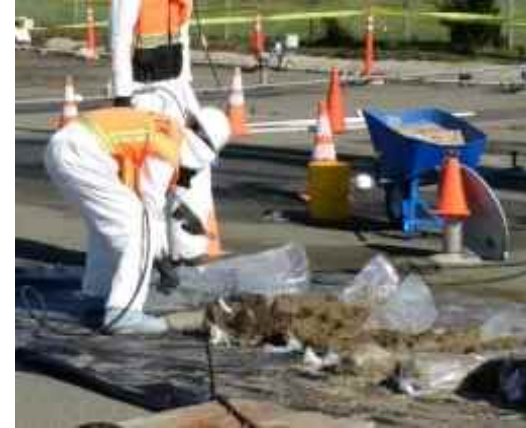
Soil Logging/Sample Collection
