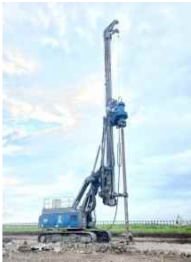
Phase 2 ISS Drilling Rig (shorter mast, less torque, smaller-diameter augers)
