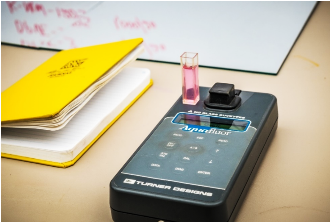
Aquafluor Meter: Measures intensity of fluorescence
