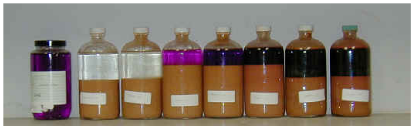
Figure 1. Sample Containers after a TOD Test with Permanganate
