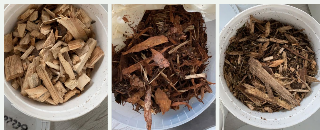
Figure 2. Hardwood mulch samples in the bench-scale test.
