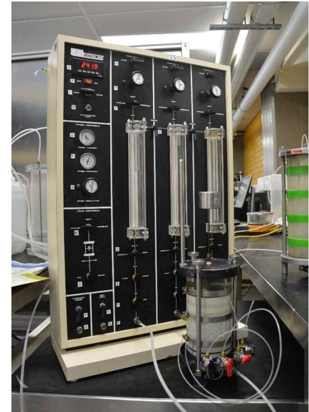
Figure 1: Schematic representation for Constant head Permeability test
