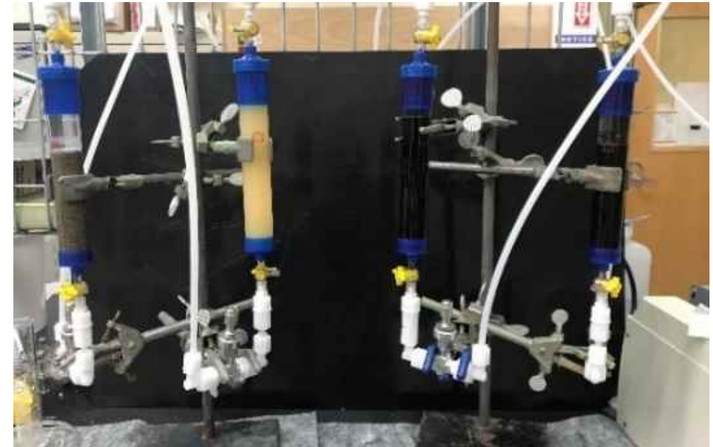
Column testing to support adsorbent media selection
