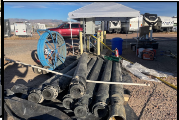
C: GAC cartridges temporarily removed
