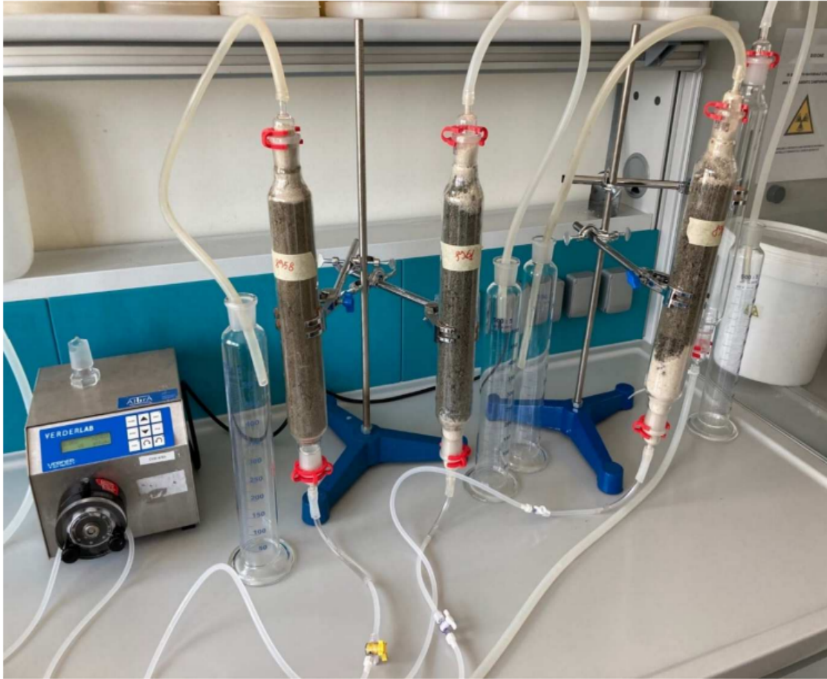
Figure 1. Column equipment for dynamic leaching test.
