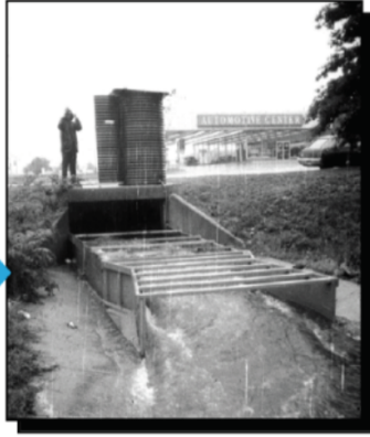
Intra-Event Runoff + PFAS Sampling at AFFF Site Discharge Point Using Automatic Samplers
