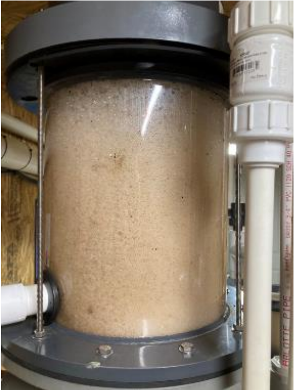
Foam Column at Top of Fractionator
