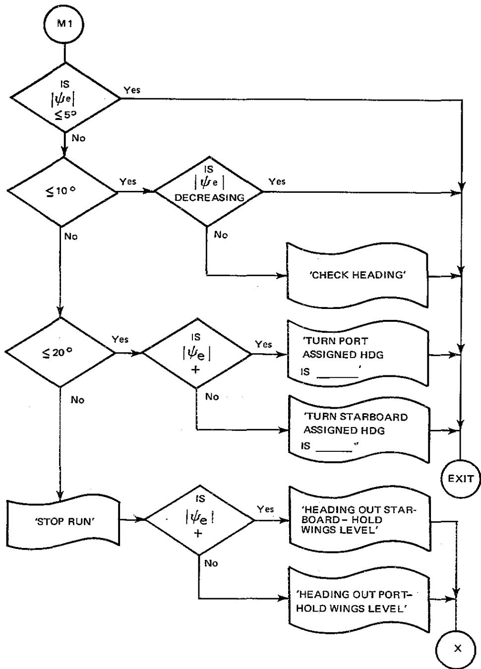
Figure 1. Heading Error Monitoring Module
