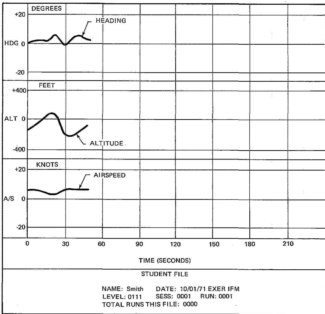
Figure 2. Typical Instructor Display of Parameter Errors
