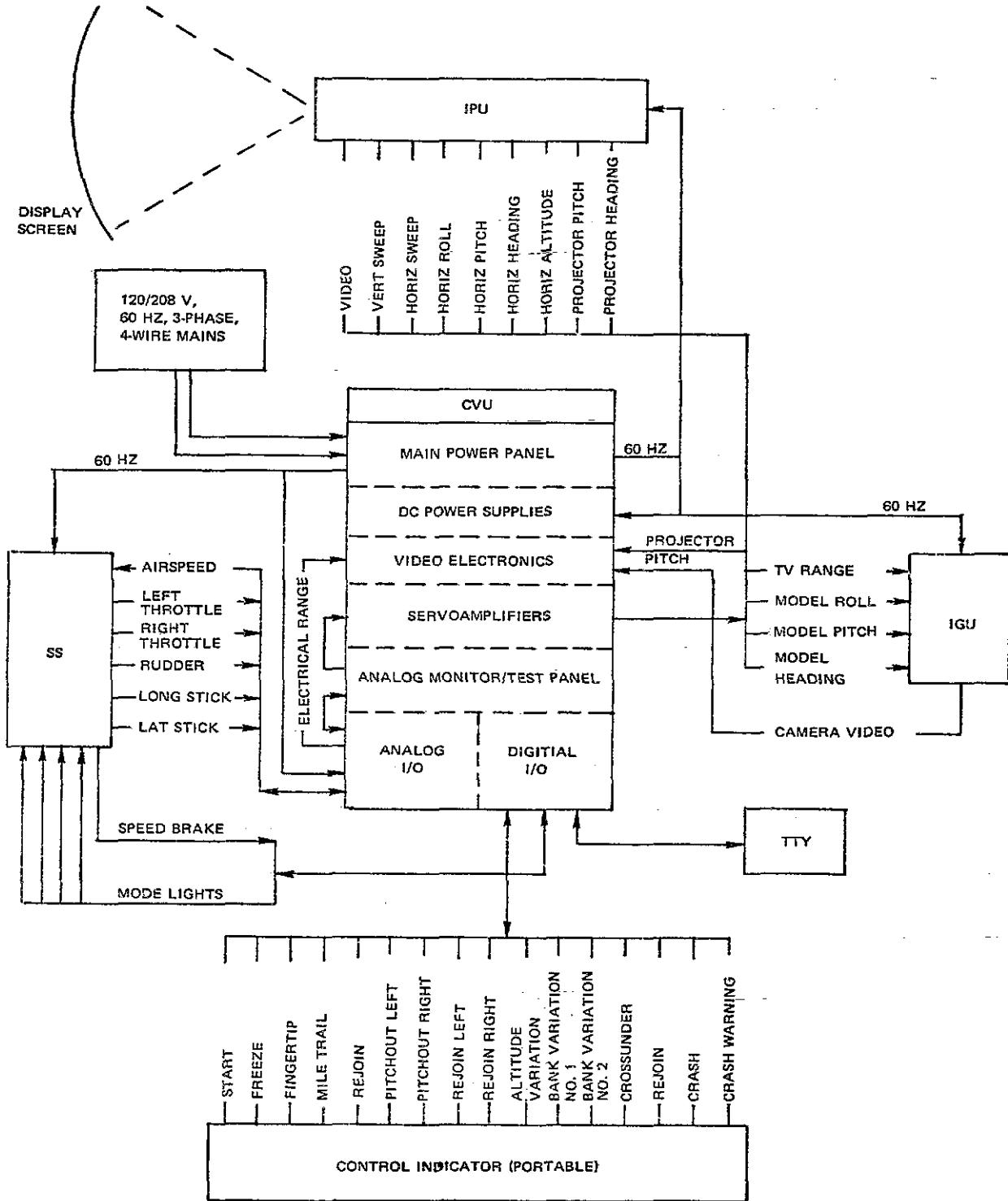
Figure 3 - System Electrical Interconnections
