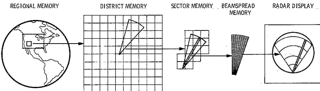
Figure 3. Memory Hierarchy of the Digital Radar Landmass Simulator
