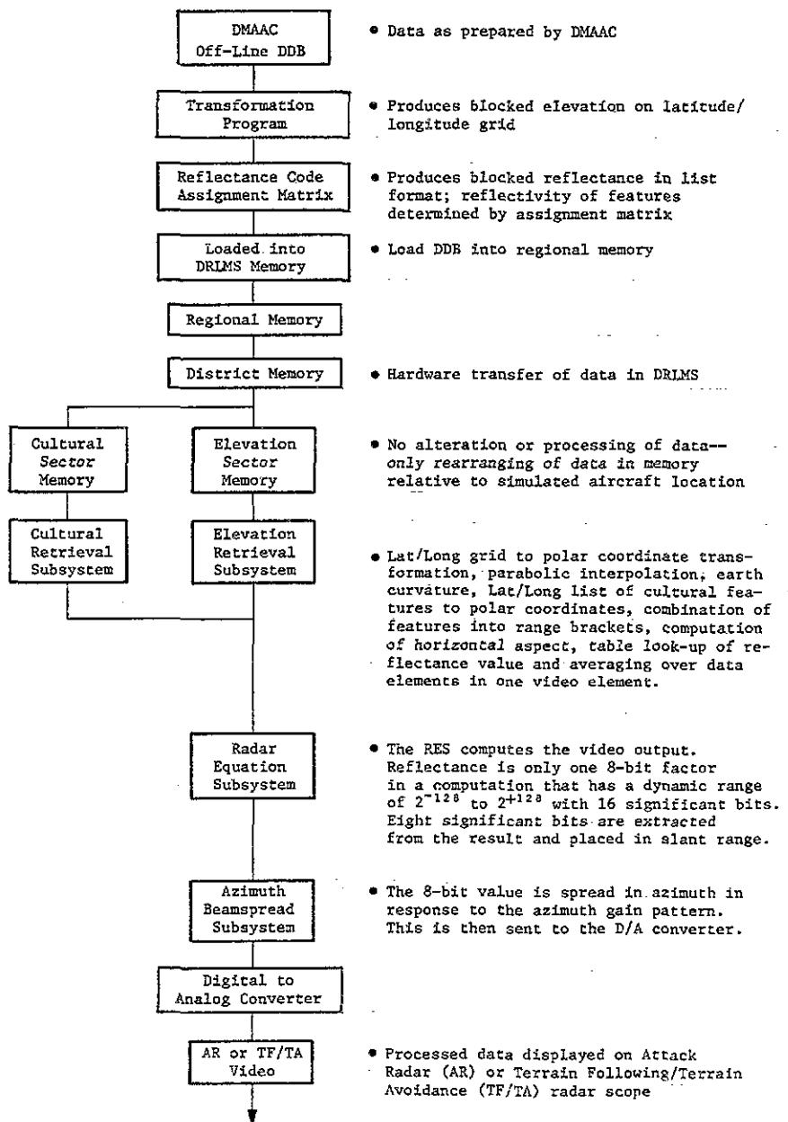
Figure 2. Data Path Flow Chart - DMAAC to the Radar Display
