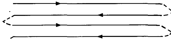
d. Write on Retrace-Y Properly Damped
