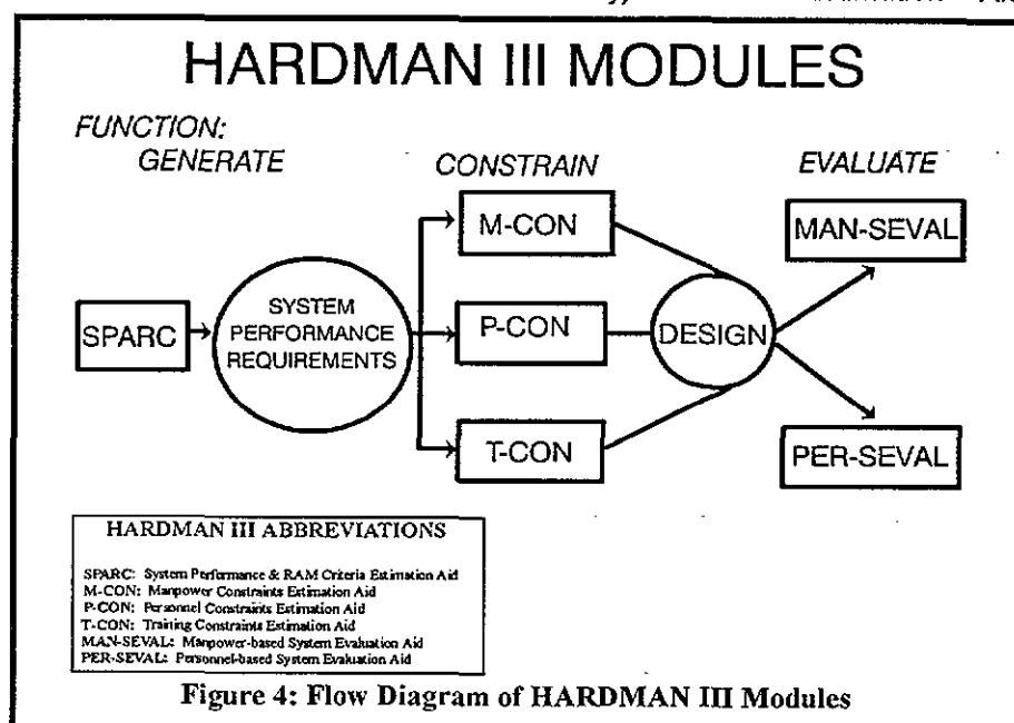
Figure 4: Flow Diagram of HARDMAN III Modules
