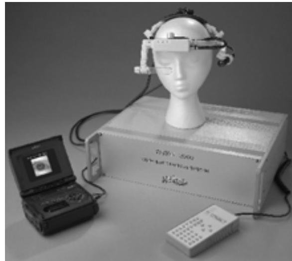
Figure 2. Components of the El Mar, Inc. Vision 2000 Portable Eye Measurement System. From Left to Right, The 8 mm VCR and Display, Headband With Eye Tracker Sensor and Side Mounted Scene Camera, The Main Processor and Hand Controller Unit.
