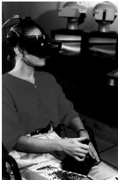
Figure 3. Student with helmet-mounted virtual reality display.
