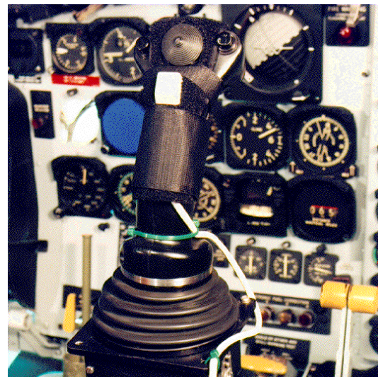
Figure 3. Tracking sensors are easily attached to control sticks in a typical aircraft cockpit.
