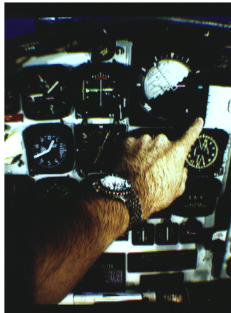
Figure 7. Image layering capability, with correct foreground-to-background ordering. Note that pilot can read his own wrist watch with VEDS.
