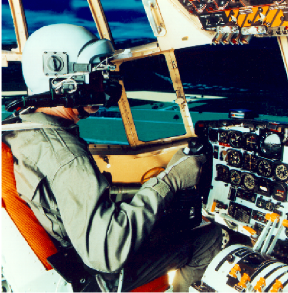
Figure 2. Actual HMD image as seen by pilot using VEDS system.
