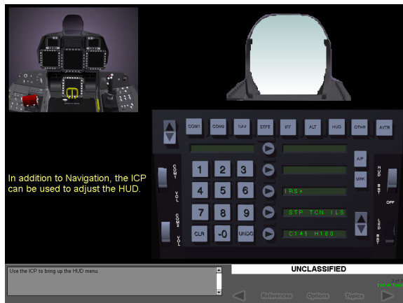
Figure 9. F-22 ICP Dual Mode Smart Graphic in Simulation Mode
