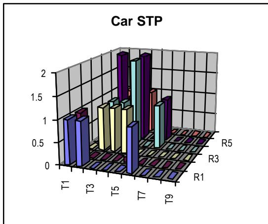
The costs related to the vehicle handling and traffic interaction are clearly visible (R1, R4, R5). The high relative costs of the image generation are reflected by the fact that the row T4 is relatively high populated. The limited training aims and flexibility in training clearly show up in the missing components for exercise evaluation and generation (T7, T8).
