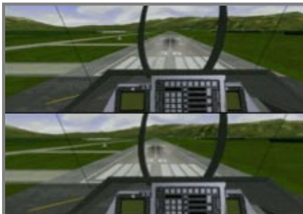
Figure 7. Upper image shows head movement to the left without Virtual Collimation. Lower image shows the same movement with Virtual Collimation resulting in real-world parallax effects.
