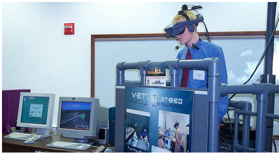
Figure 1: Photo of equipment for running VETT. Note HMD with head tracking unit on top and microphone on the subject, with monitors in the background. Not shown: 2 CPUs located beneath the monitors.
