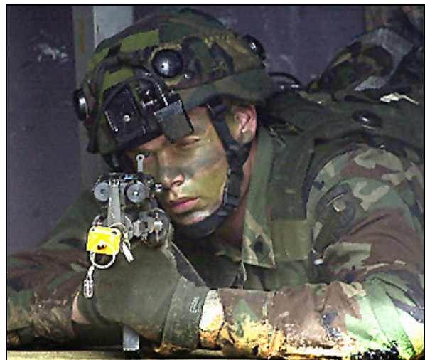
Figure 1. The Land Warrior concept demonstration (taken from Graves, 2001). The helmet is configured with a monocular display and cameras with the capability to stream video and thermal imagery during reconnaissance operations.
