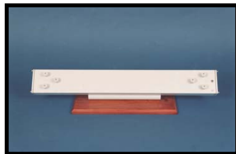
Figure 7. Two Cluster Target Scoring Bar (TDCue™ Model 2F2S) with 6 Sensing Elements.
