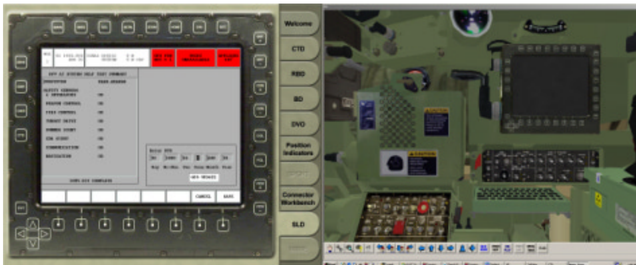
Figure 6: The M2A3/M3A3 VR DT uses a combination 3D and 2D displays where the 2D display is driven directly by the tactical software.
