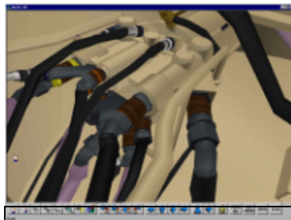
Figure 4: The M270A1 VR DT has detailed 3D VR models of the hydraulics system for the missile launcher loader.
