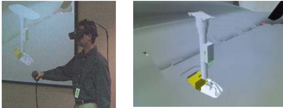
Figure 1. (a) Participant using the immersive visor and 3-D mouse; (b) View of the maintenance task from within the visor.
