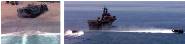
Figure 2. Left: An LCAC transports cargo and troops to a secure beach site. Right: Two LCACs depart an Amphibious Transport Dock (LPD).
