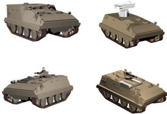
Figure 4. Common Chassis, Four Different Systems
