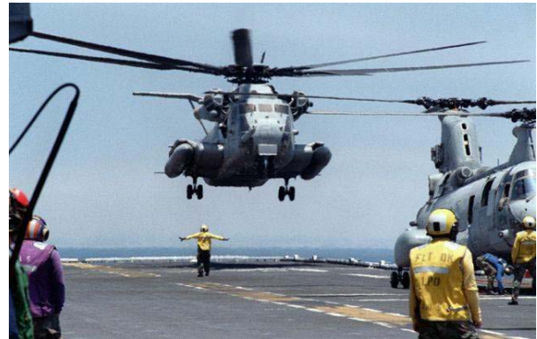
Figure 1. LSE signaling a helicopter aboard ship. The LSE standing in front of the helicopter in the center of the picture is giving the Hover signal.
