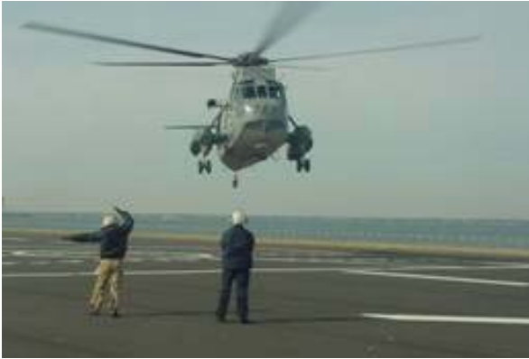
Figure 2. Supervised LSE signaling training during a live practice pad session. The student (left) is giving the “Move Right” signal under instructor supervision.
