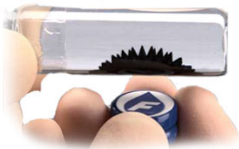
Figure 6. Ferrofluid moves according to the magnetic flux lines as shown
