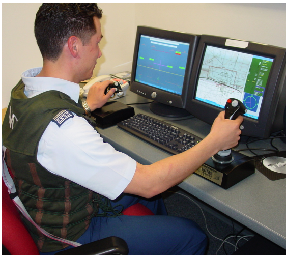
Figure 2. TNO vibrotactile vest as implemented with the UAV STE in the vest condition.
