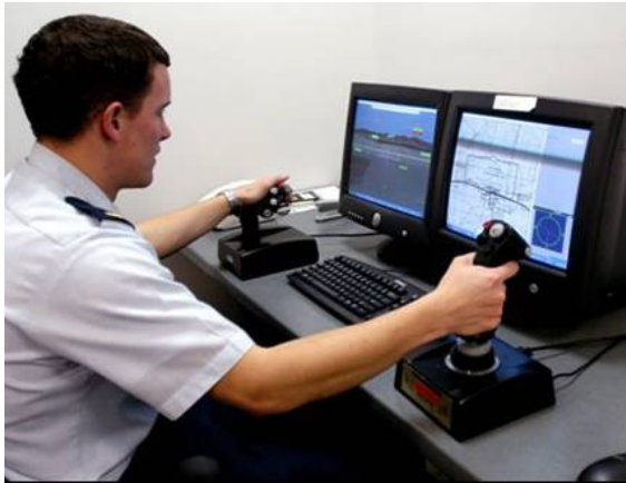
Figure 1. UAV STE with hands-on throttle and stick (no vest condition).
