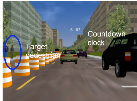
Figure 1. Image from driver's forward view, with a countdown clock, slow lead vehicle, target pedestrian, and parked vehicles.
