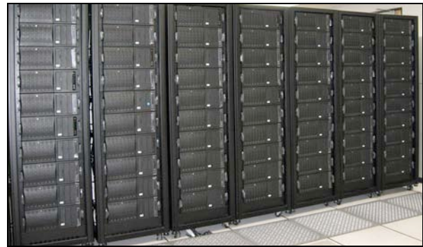
Figure 1. Joshua cluster at JFCOM consisting of 256 dual quad core Opteron processors and 256 NVIDIA GTS8800 GPUs (Photo Source: Ed Aaron, USJFCOM).
