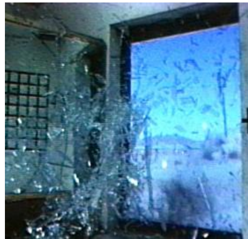
Figure 3 Injuries from glass breakage is one example of an effect that can not be accurately modeled using pre-calculated results
