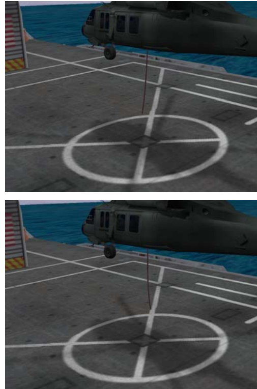
Figure 13. Snapshots from CHARM/ODE Engine Modeling Rotorwash Effects on Flexible Cable
