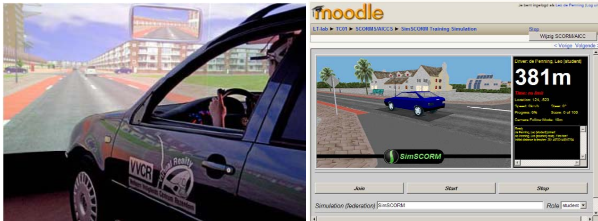
Figure 5. The SimSCORM demonstrator with an HLA compliant driving simulator (left) and a Moodle-based student interface (right).
