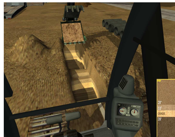
Figure 5: Shadows, trench coloring and gauges enhance depth perception
