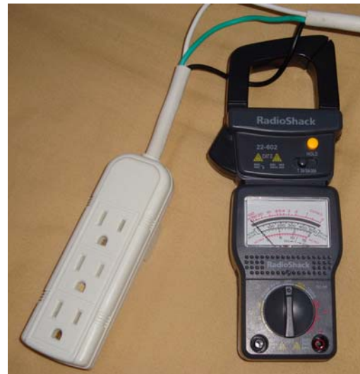
Figure 3. Image of the Ammeter used for Current Testing
