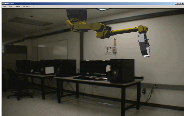
Figure 1. The DRSS uses the virtual prototype of a gantry robot arm and augmented reality to demonstrate the functions of the safety system.
