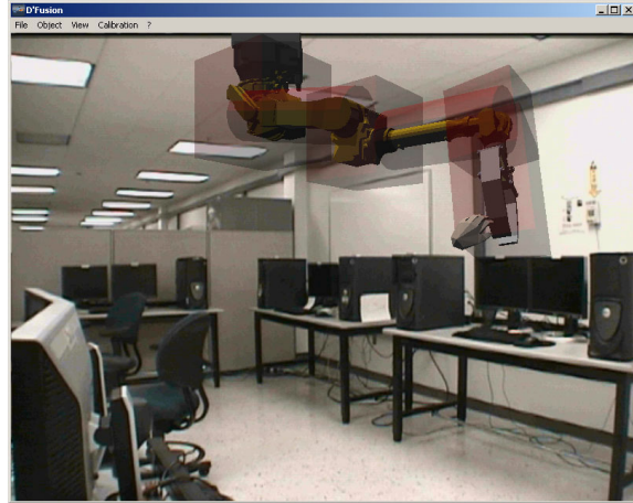
Figure 7. When the red light (danger) is on, the DRSS controller starts the sirens and sets the brakes to all robot drives. The human operators can see the red light when using special goggles.
