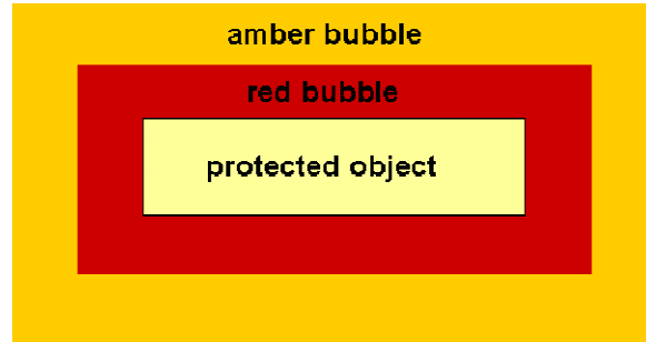
Figure 2. The simple cross-section view shows the concept of using two imaginary bubbles to wrap around the protected object. The amber bubble indicates caution; the red bubble indicates danger.
