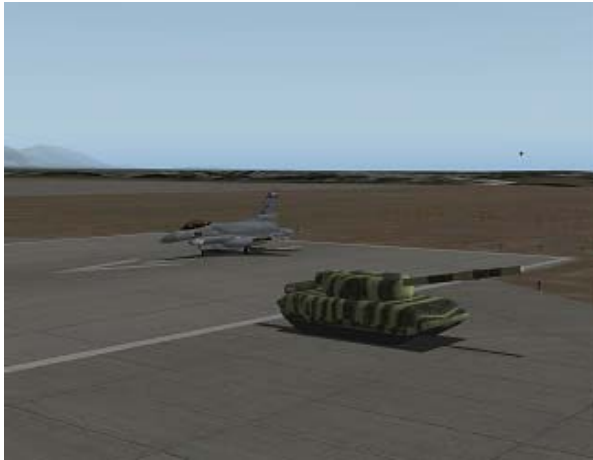
Figure 7. Implementation of Ground Clamping Algorithm to Eliminate Vertical Correlation Error for Entity Position (Foreground Tank) Received Via DIS Network.
