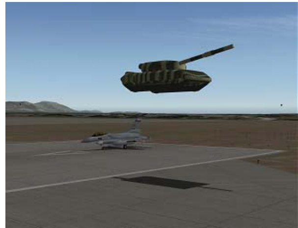
Figure 6. Correlation Errors Between Native X-Plane® Entity Position (Background F-16) and XCITE Entity Position (Foreground Tank) Received Via DIS Network.
