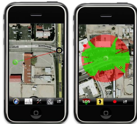
Figure 1. LOS capabilities of the iPhone app. The left image shows a point-to-point LOS query that is blocked by a building. The right view shows a 360 degree field-of-view LOS with various areas of clear (green/lighter shade) and blocked (red/darker shade) LOS.
