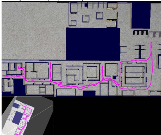
Figure 10: Real-time computed camera trajectory corresponding to a 253.82 m run over 5.64 minutes
