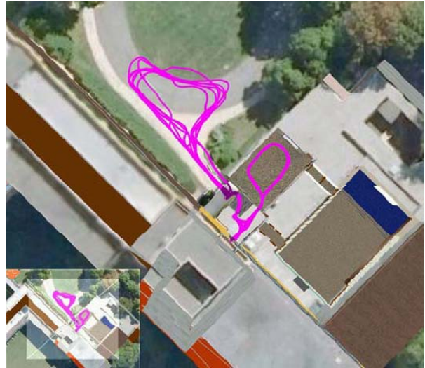
Figure 8: Real-time computed camera trajectory corresponding to an 810 meter path completed in 16.4 minutes during a live exercise.
