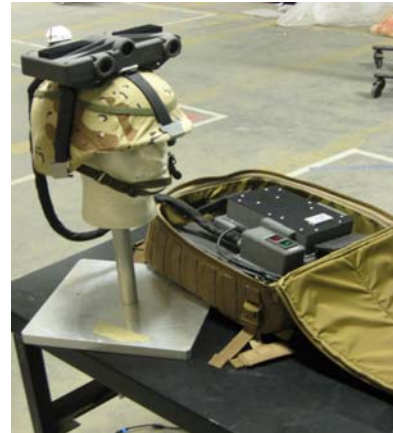
Figure 1: Helmet with forward and backward facing stereo cameras and MEMS IMU and ruggedized laptop processing units shown in back-pack.
