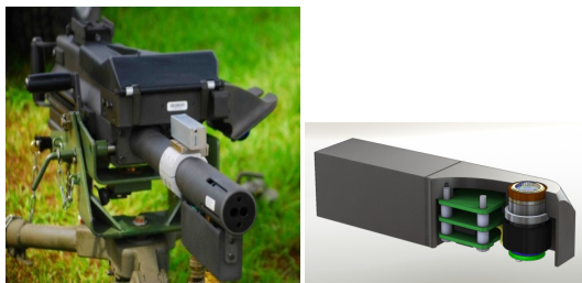
Figure 4 – Prototype WOM Sensor
