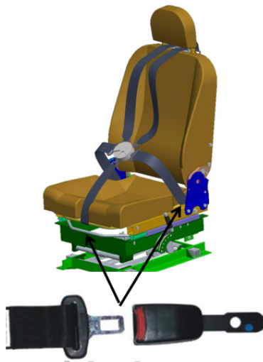
Figure 3. Reconfigurable Seat Restraint Design
